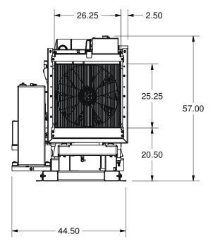
\* This is the width of the machine with the fuel tank and controller enclosure removed
